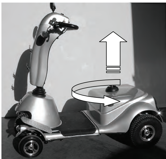
To remove the seat pull the revolving seat lever up, turn the seat & lift. (Caution this is heavy) Remove the rear cover by lifting upwards. This is attached with Velcro
