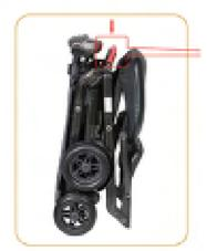
Push down the carry handle as far as possible and the scooter will start to unfold.
