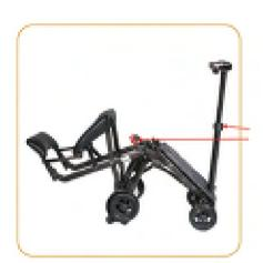
Use one hand to hold the tiller and the other to hold the handle or bottom of the seat to guide the scooter apart.
